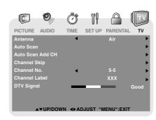
Antenna : Air (over-the-air broadcasts, Ch 2-69) or CATV (cable/satellite broadcasts, CH
